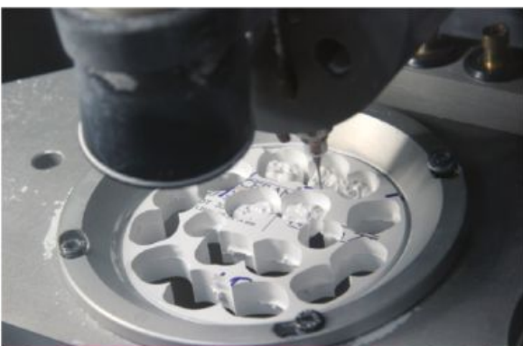
Precise industrial milling of a zirconia block.
